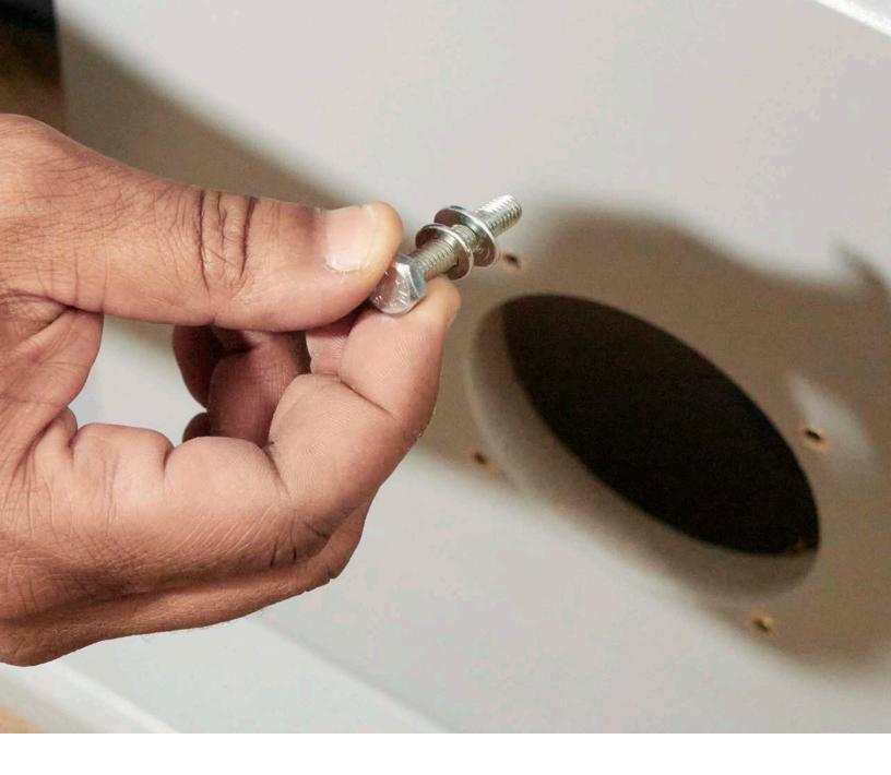
7. Using the short 1/4"- 20 bolts and washers from page 4, align the base woofer module and the base platform so the bolts drop into the threaded nut inserts. Hand-tighten only.
