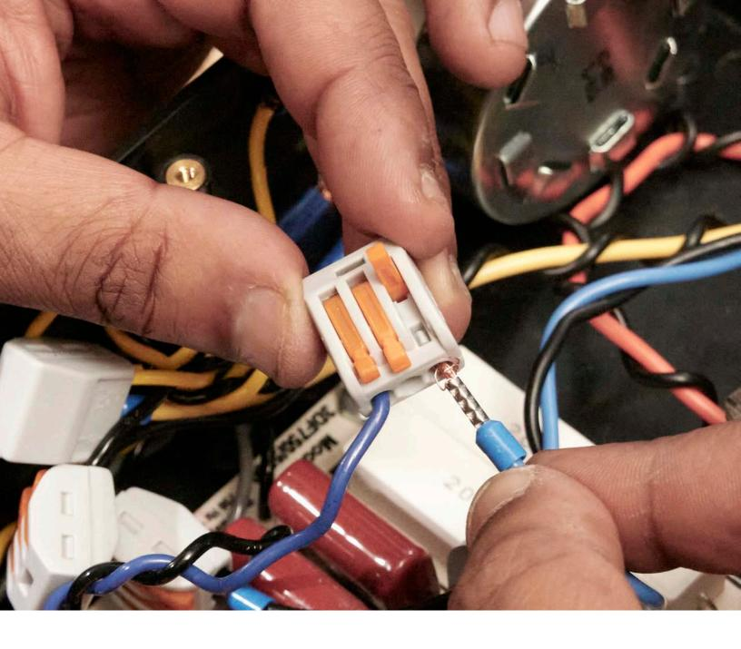
32. Crossover Network. To attach the wires to the crossover network box, cock the orange connector levers back. Match up the colorcoded wire connection slots and colored wires, and insert wires.
