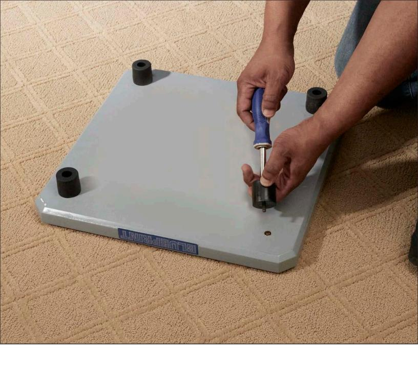
3. Feet. Locate the feet and fasteners. Align and screw the fasteners into the threaded nut inserts in the bottom of the base platform. Then turn the base platform upright.
