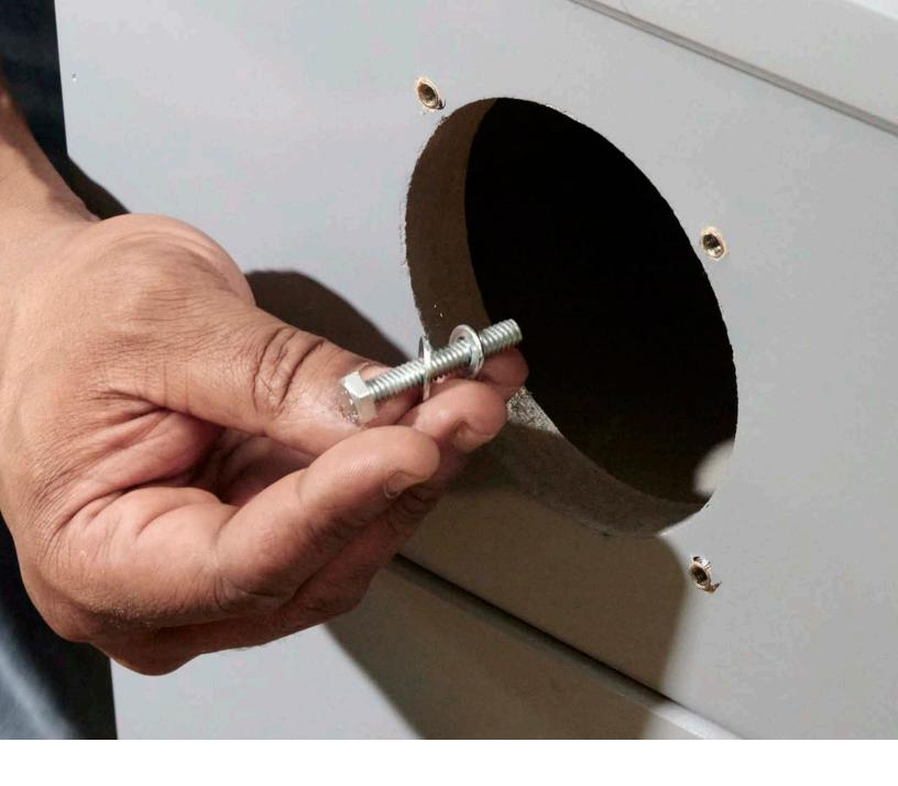
18. Slide the lock washers onto the bolts first, then the flat washers. Align the cap platform atop the top module. Insert bolts and washers into the cap platforms' threaded nut inserts. Hand-tighten.
