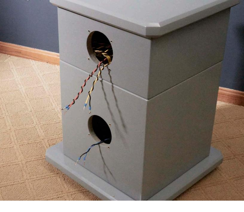
20. Wiring. Carefully unwrap and remove the three twisted pairs of wires from inside each module.
