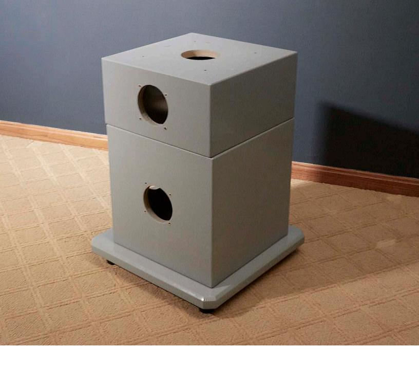
9. Stack and align all the modules. After everything looks aligned, properly go back with the wrench and tighten down the bolts that connect the base woofer module to the base platform.
