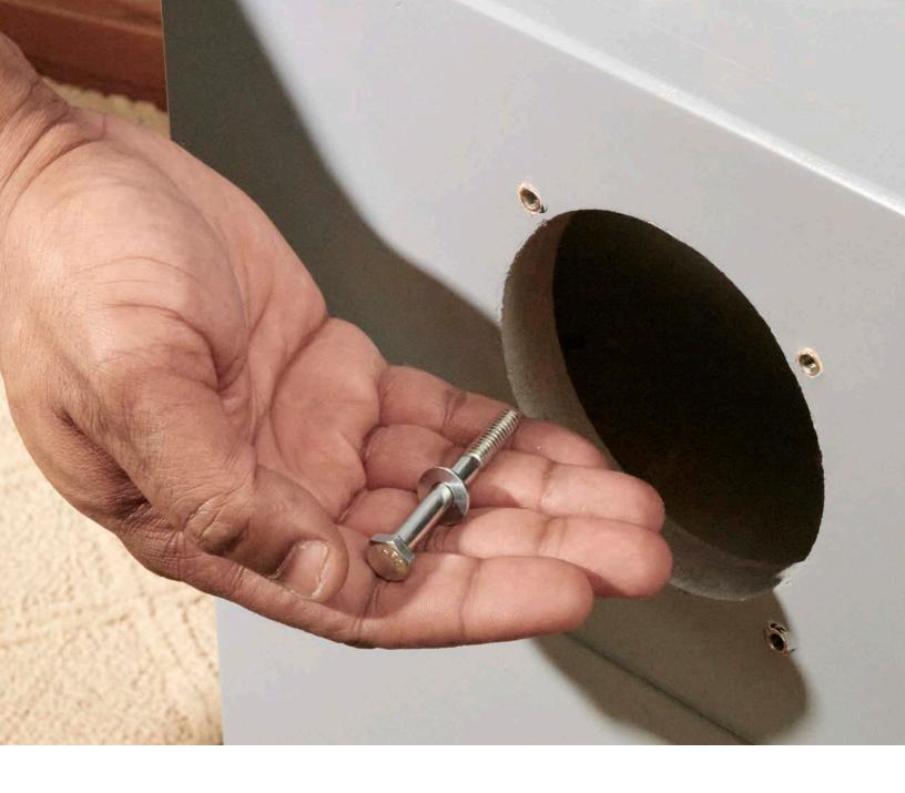
11. Slide one flat washer onto each of the long 1/4"-20 bolts.
