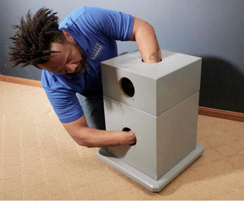
16. Using both wrenches, one on the top and one on the bottom, snug down the four bolts that hold the two modules together. Do not bump the upper module and knock it out of alignment.
