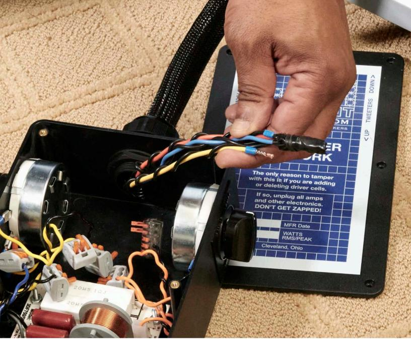
25. Pull the wires through the tube so that 8" of wire protrudes into the crossover network box. Crossover instructions will commence on pages 32 and 33, after Plug Option and Back Caps.
