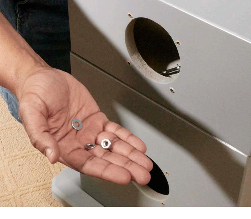
14. Locate the downward protruding bolts. Put the flat washers on first, then the lock washers. Then hand-thread the nuts onto the bolts.
