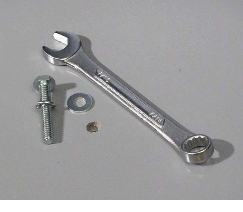
4. Modules. Locate four short 1/4"- 20 bolts, four lock washers, and four flat washers. Lock washers go on first, then flat washers. Bolts will go into the threaded nut inserts in the top of the base platform.
