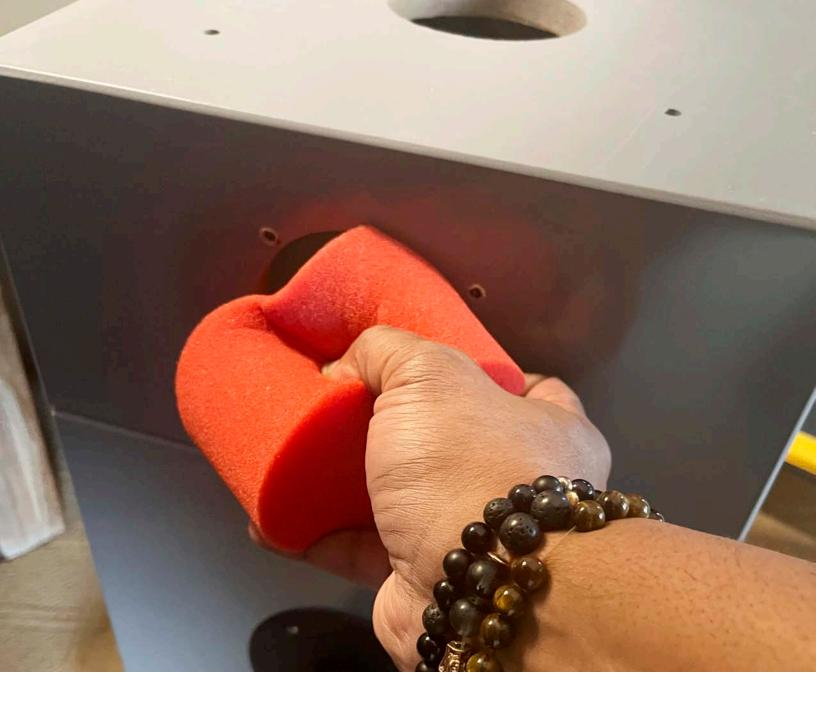
27. Insert the compressed foam plug into the module, and insert it carefully into the holes between modules. Be careful not to pull any of the wires.
