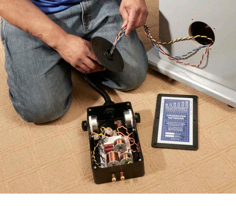
24. Fish the three twisted pairs of wires into the plastic/foam tube and into the crossover network box.
