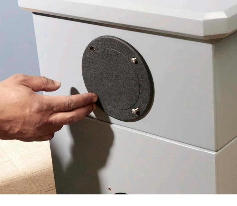
29. Back Caps. Find the small black machine screws (silver screws shown here) and hand-thread them through the black plastic back caps onto the backs of the modules.
