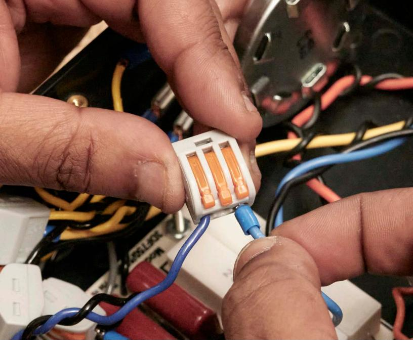
33. Insert the colored wires fully into their corresponding color-coded slots, then fully close the orange connector levers.
