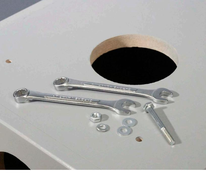
10. The subsequent stacked modules above the base woofer module require the long 1/4"-20 bolts to attach to each other. Each bolt utilizes one lock washer, two flat washers, and one nut.
