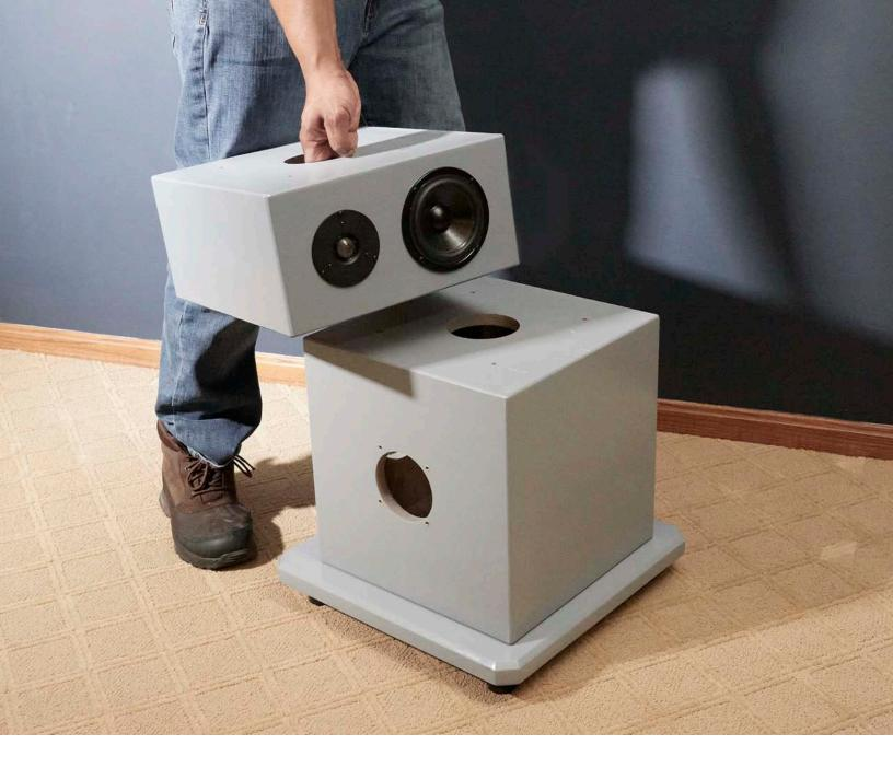
8. Unpack the next stacked module. Set it on top of the base woofer module. Align so that the drivers face the same direction. Repeat page 8-19 instructions for all additional stacked modules.
